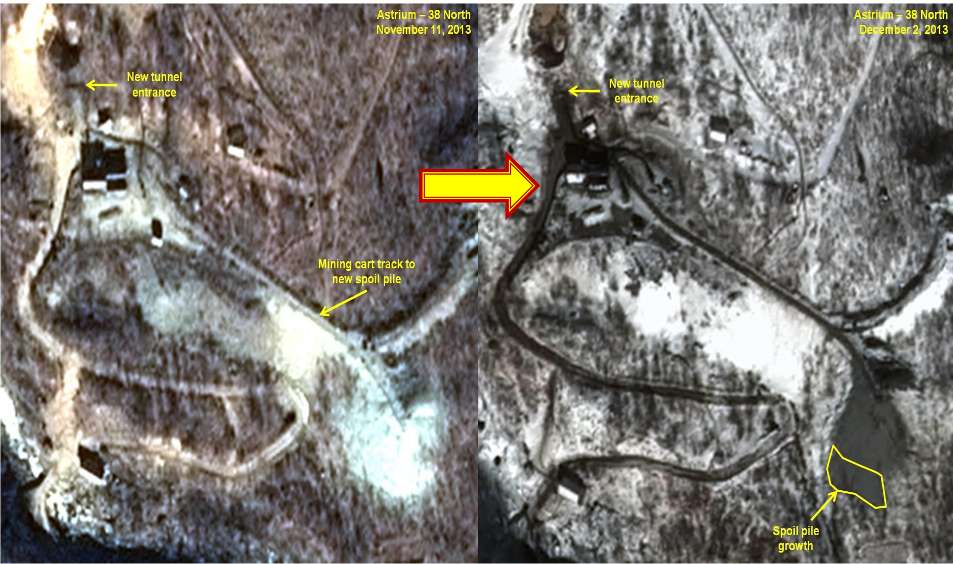
Figure 5. West Portal Activity – Tunnel Excavation and Spoil Pile Growth (November 11, 2013 and December 2, 2013)
